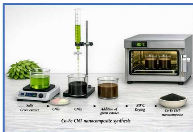
Fig. 1. Schematic illustration of the biosynthesis process for the MK leaf extract-mediated CNT-Co-Fe (2.5 wt% and 5 wt%) nanocomposites.
